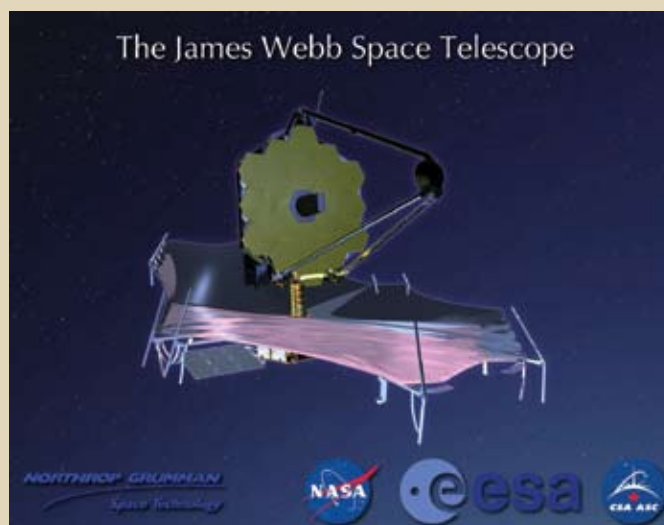
Figure 3 Scheduled for launch in 2011, the James Webb Space Telescope (JWST) is a new, larger successor to the Hubble Space Telescope. Shown here is an illustration of the JWST as it will be deployed. The gold-coated telescope mirror is shown at the top of the picture, the purple sunshield at the bottom.
